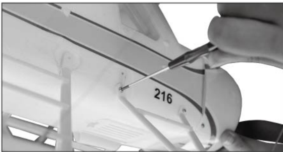
21 Fasten the float brackets to the fuselage with PA2.5*8mm screws.
