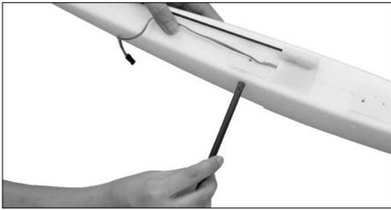
17 Connect the floats with \varnothing 8 \times 359 mm glass fibre tubes.
