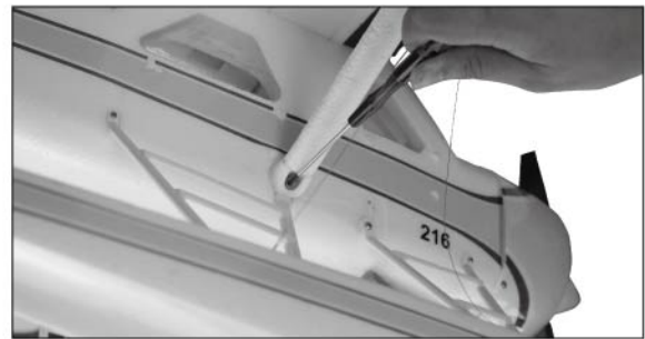
22 Fix wing struts and floats with PA2.5*8mm screws.
